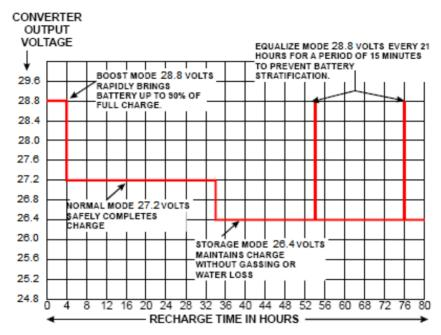
**28.8 Volts (Boost Mode)**Rapidly brings the batteries up to 90% of full charge / LED is steady ON
